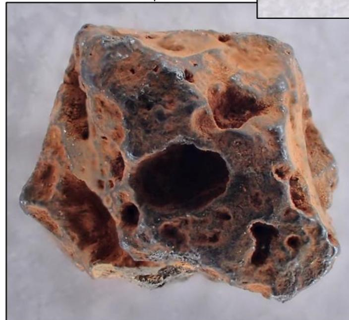
Enlarged photos of external appearance of fuel debris sample (taken from directly above)
