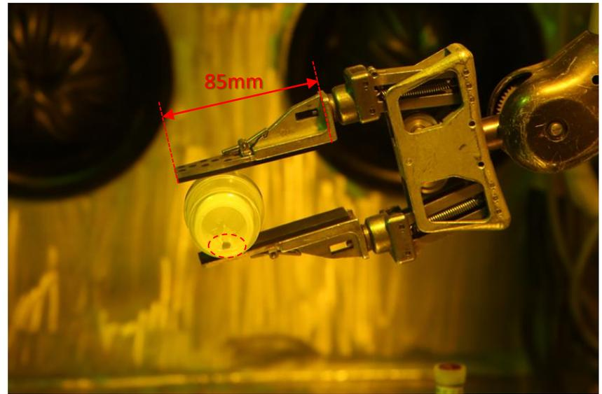
Fuel debris sample inside a specimen container
