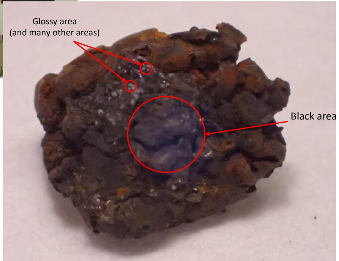
Enlarged photo of External appearance of fuel debris sample
