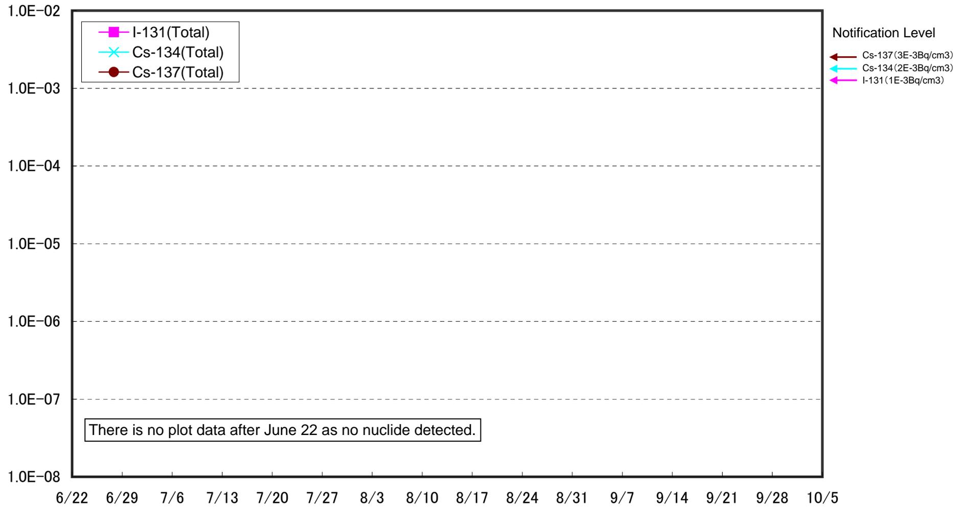
Dust Nuclides Analysis Results at Unit 1 North Side Slope at Fukushima Daiichi NPS (Bq/cm<sup>3</sup>)
