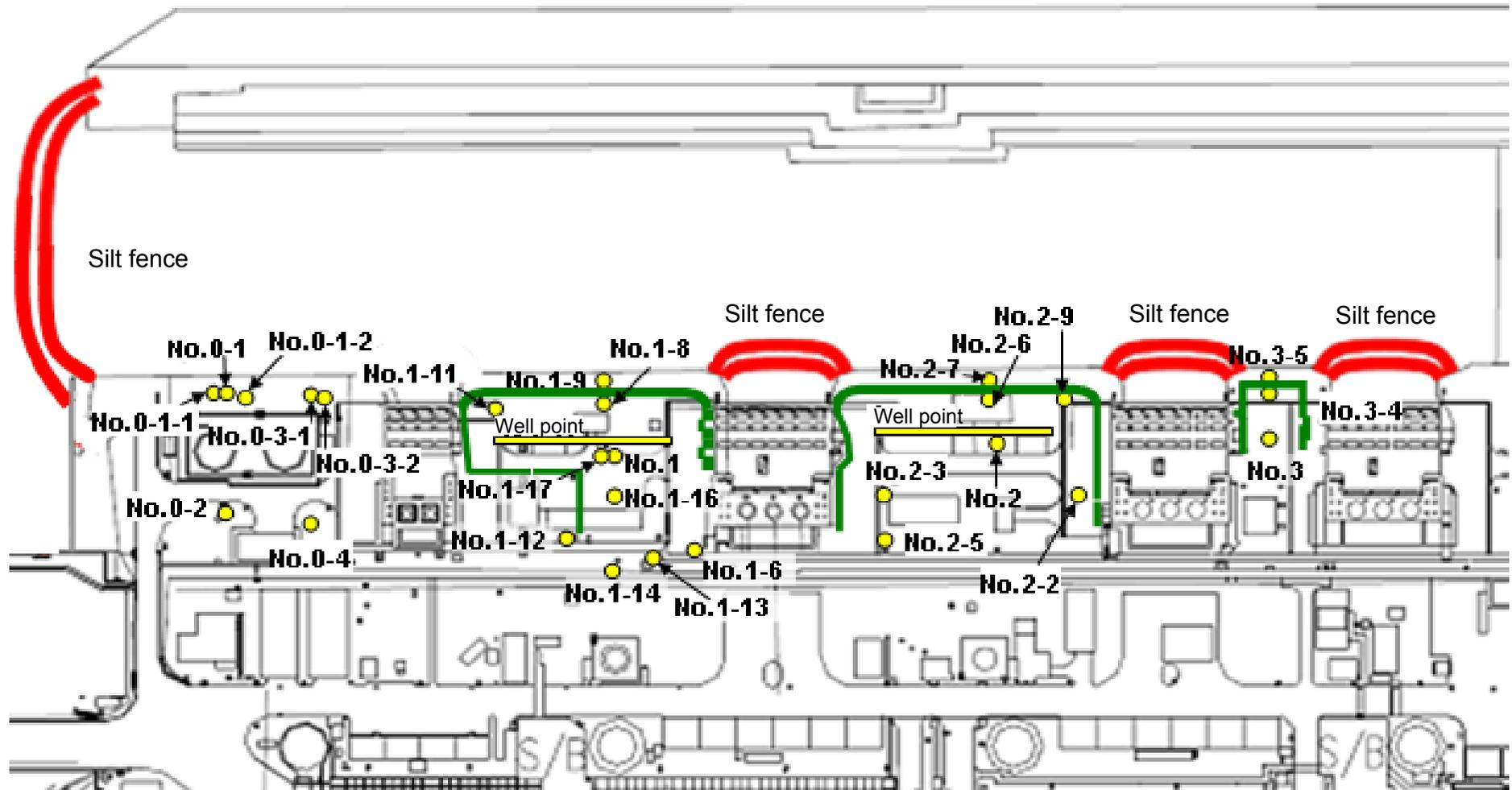
— : Location where ground improvement construction was completed, or being implemented (as of January 31, 2014)
