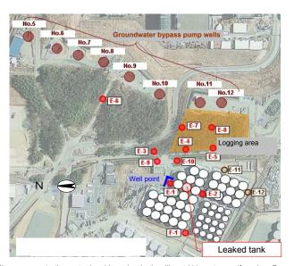
%In response to the water level lowering in the dike at H4 east area (found on December 24, 2013), the groundwater observation holes E-11and E-12 will be additionally established, in order to investigate the influence of leak water on groundwater
