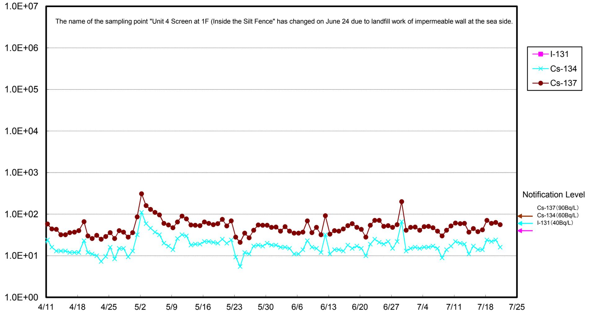
Radioactivity Density of the Seawater at the South of Unit 1-4 Water Intake (in front of Impermeable Wall)
