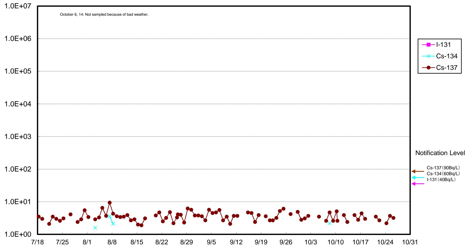
Radioactivity Density of the Seawater at the North of Unit 1-4 Water Intake (North of East Seawater Break
