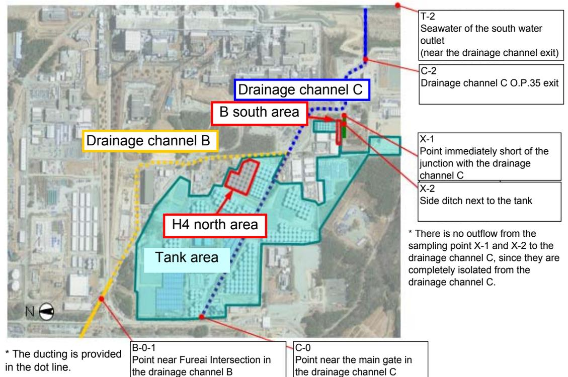
\* There is no outflow from the sampling point X-1 and X-2 to the drainage channel C, since they are completely isolated from the drainage channel C.
