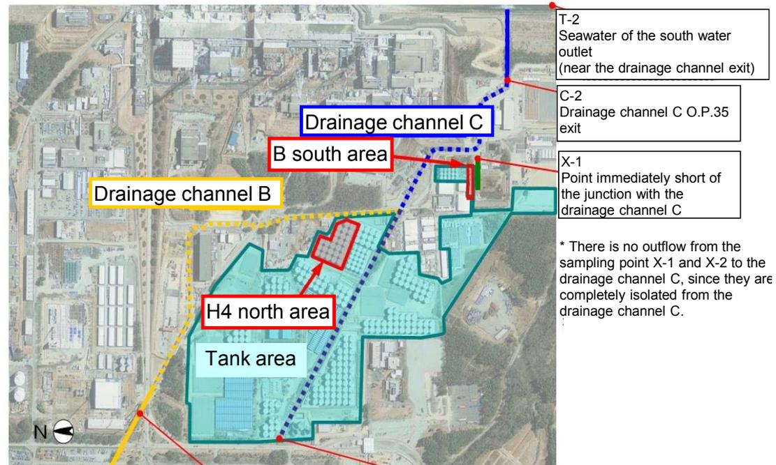
\* There is no outflow from the sampling point X-1 and X-2 to the drainage channel C, since they are completely isolated from the drainage channel C.
