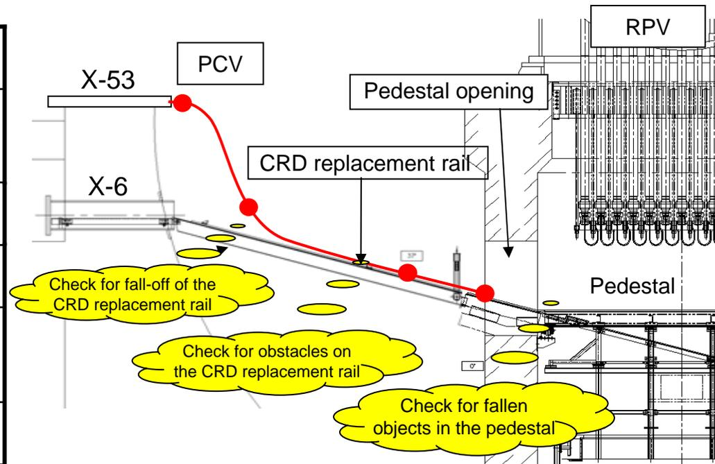
Scope of investigation of the inside of the PCV to be performed through X-53
