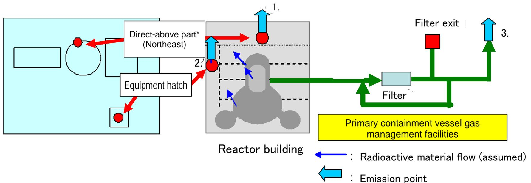
\* Depending on situation, we conduct the sampling at several points on the operating floor, and adopt a point with the highest dust density as the representative point of the directly above the operating floor part.
