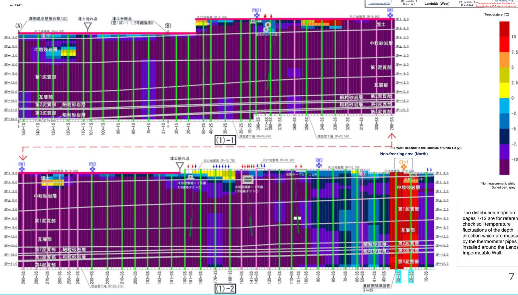
The distribution maps on pages 7-12 are for reference to check soil temperature fluctuations of the depth direction which are measured by the thermometer pipes installed around the Landside Impermeable Wall.
