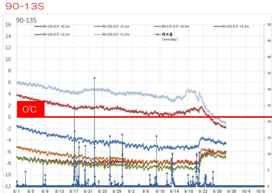
\*The soil temperature at 90-13S fell below 0°C. However, the soil temperature at the adjacent 80-13S rose. Groundwater flowed into 80-13S because it lost paces to go due to the success of supplementary method for 90-13S. Therefore, application of supplementary methods at 80-13S continues.
