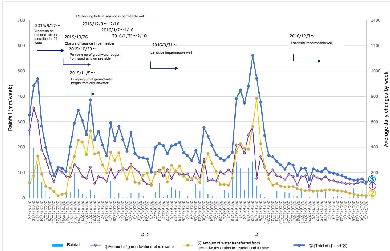
mount of water transferred from groundwater drains to reactor and turbine building
