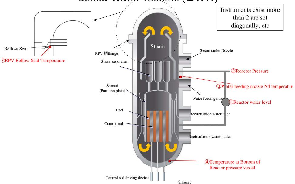
Cross section of Primary Containment Vessel Boiled Water Reactor(BWR)
