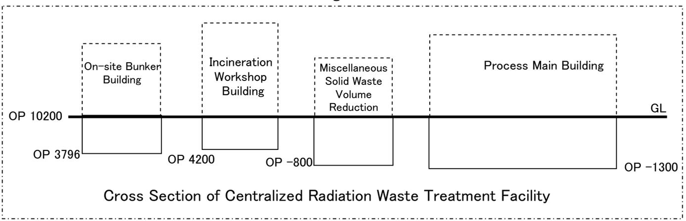
Cross Section of Centralized Radiation Waste Treatment Facility
