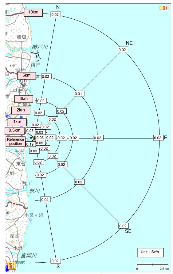
We measured by NaI scintillation survey meter on a ship.
