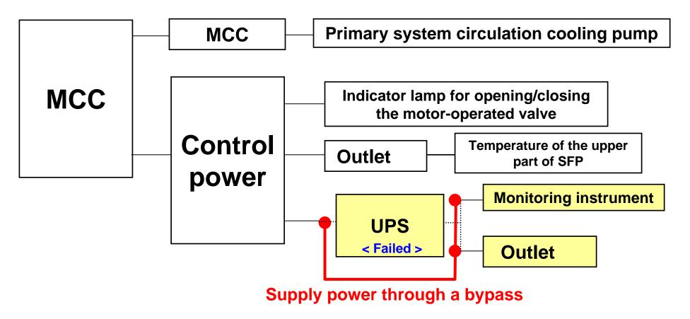
Upon investigation, it was confirmed that a system trip occurred as a result of UPS failure causing the loss of power supply to the monitoring instrument. The cooling system was recovered by supplying power to the monitoring instrument through a bypass. After replacing the failed UPS, power supply through UPS will be recovered.
