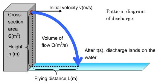
Based on the flying distance and height, assuming discharged liquid in falling motion, volume of flow is calculated as follows:
