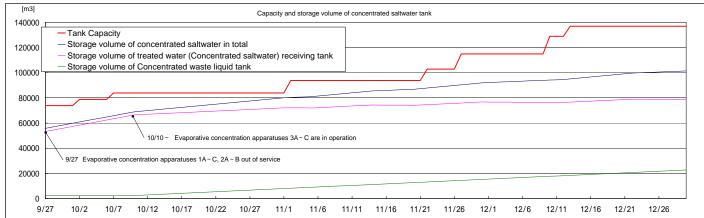
注記 - Amount of water treatment is assumed to be 1320m3/d (It can be adjusted according to level of accumulated water in T/B.)
