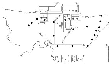
Location of seismometers on the ground surface in the site
