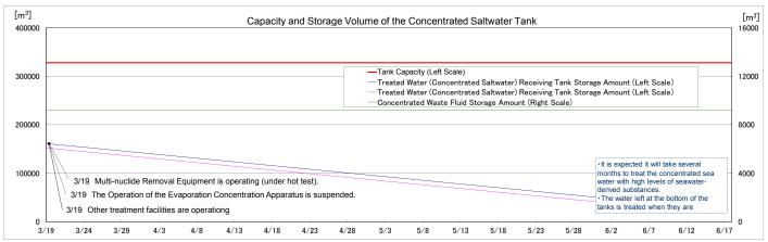
The treated water volume is assumed to be 720m³/d (Subject to change depending on the level of water accumulated in T/B).
